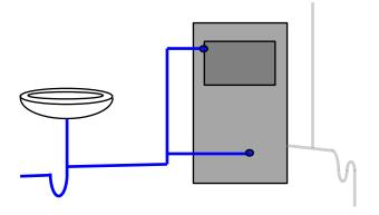
C: Typical connection to single drain system
