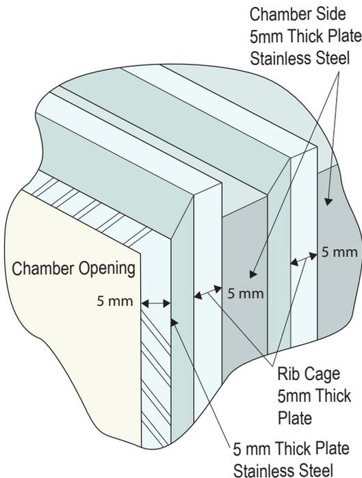
The amount of energy required to bring all that steel up to 121°C – the vessel and the rib cage – and hold it there, for any period of time, is enormous. To complicate matters further, in order to provide the high-throughput hospital operations demand, an additional steel box encases the rib cage. By keeping this so-called “steam jacket” hot between cycles, operators can bring the pressure chamber up to sterilizing temperature more quickly.
