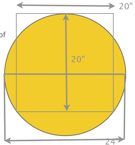
It's as simple and irrefutable as any law of physics: A lighter chamber is more efficient, heats faster, and consumes far less energy in the process. For similar sterilizing cycles with similarly sized chambers, a cylindrical research-grade autoclave will always outperform its rectangular medical-grade counterpart.
