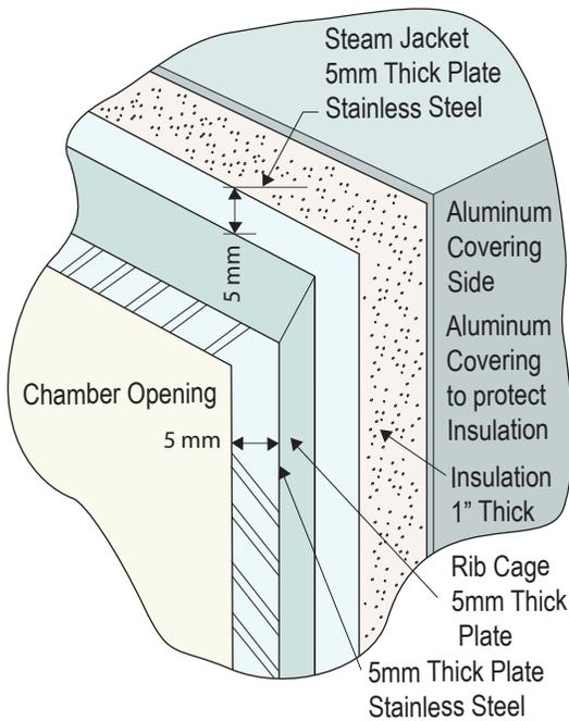
But putting a second cube around the first cube does nothing to address the challenge of keeping such an incredible mass at 121°C. Most manufacturers address this issue by wrapping their double-walled steam box with an insulating blanket.
