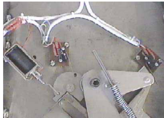
Locking Solenoid & Micro-switches - Detail
