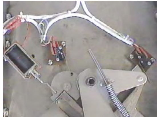
Locking Solenoid & Microswitches - Detail
