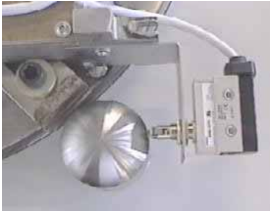
Door Closed Microswitch - Detail
