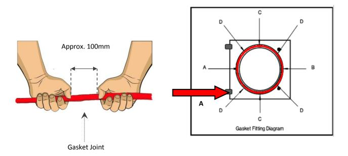
Find the opposite centre line of the gasket and press firmly into the point marked **B** on the diagram, ensure that there is an even amount of gasket each side of points **A** and **B**.
