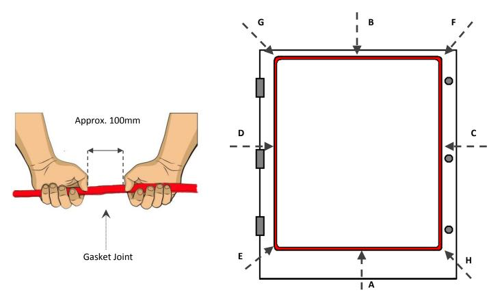
Find the opposite centre line of the gasket and press firmly into the point marked **B** on the diagram, ensure that there is an even amount of gasket each side of points **A** and **B**.
