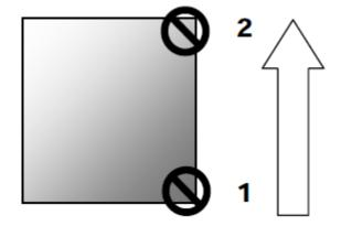
**3.** Open the door by undoing the lower black hand-wheel first followed by the red safety handwheel. With the door free, carefully pull open.
