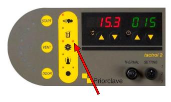
The COOLING Fan switching ON will be delayed until a pre-set control temperature is below the setting selected – Default is 100 degrees.
