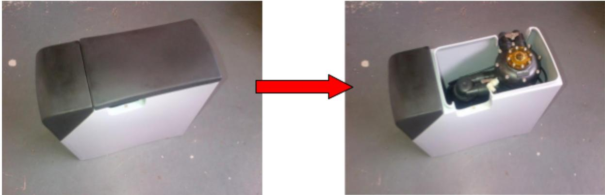
Locate adjustment screw of the regeneration unit
