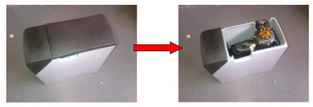
Locate adjustment screw of the regeneration unit
