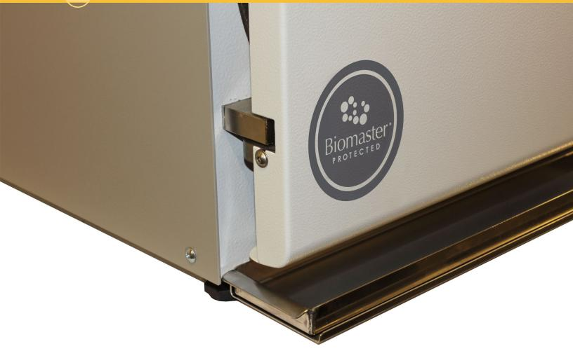
Priorclave is the only manufacturer to offer **Biomaster**<sup>\*</sup> **Protected Antimicrobial Surfaces**. All epoxy coated panels and frame members are treated with this silver-based surface coating, providing a second line of defense against cross contamination. Extensive validation through independent laboratories demonstrates that Biomaster inhibits microbial colonization, mold, and mildew. Biomaster coatings can't be washed off, and
