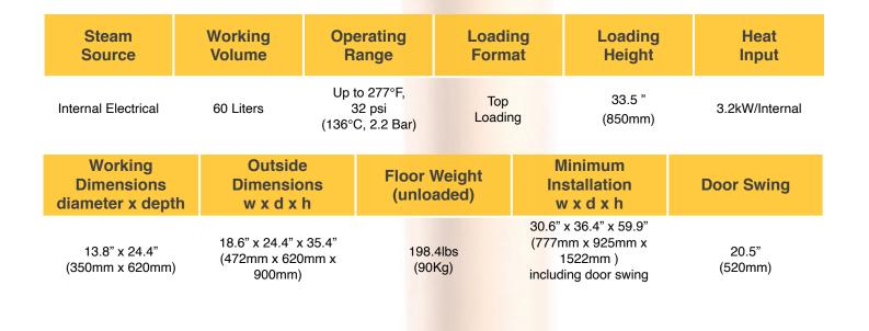
External dimensions do not include easily removable items such as door handles and outlet pipes that could be moved or removed for transport, and represent the maximum size of the machine without radical alteration.
