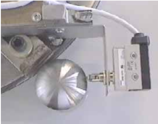
Door Closed Microswitch - Detail
