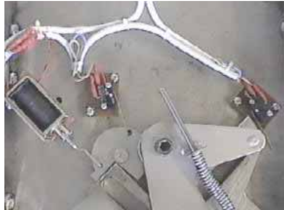
Locking Solenoid & Microswitches - Detail
