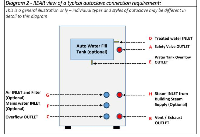
All drain piping should head downward towards the drain to prevent water collecting in the pipe.
