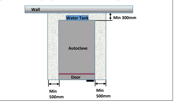
Diagram 1 - Plan view of a typical Autoclave Installation – Against a wall:
