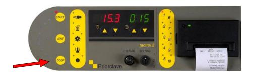
The Autoclave control system has a number of safety related features that will NOT allow the door to be opened if it is considered unsafe to do so.
